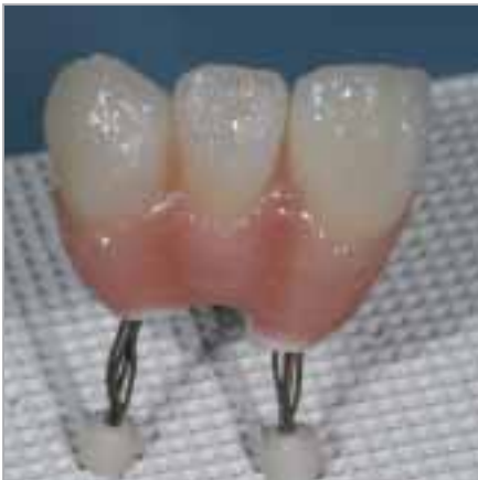
3. NobelRondo™ Zirconia Ceramics A2 and Gingiva Ceramics after baking (firing temperature 930 °C)
