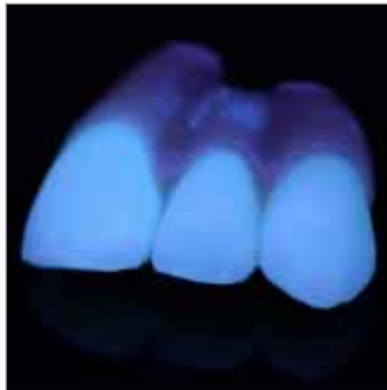
10. NobelRondo™ Zirconia Gingiva materials do not show fluorescence in UV-light
