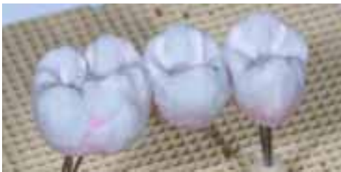
7. Procera® Bridge on Firing Tray (Final Temp. 910 °-915 °C)
